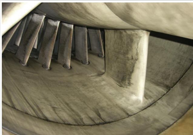
Compressor Fouling reduces energy efficiency of gas turbine engines, increases fuel consumption and CO 2 emissions.
